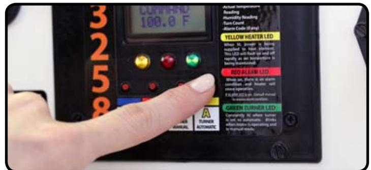
4. Press the "A" button to turn off automatic mode and allow the "M" button to function. Level the turning racks in the incubator by using the controls of the DIGITAL COMMAND CENTER. Press and hold the white M button until the racks move to a level position and then release. Racks may now be accessed. Press the yellow A button to return the incubator to automatic turning mode.
