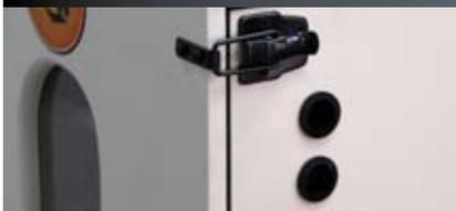
There are two holes in the upper back panel and two holes in the upper right side near the door. These holes are covered with a plastic plug. One plug on the right side and one on the back has a hole punched in them. This is to provide the necessary flow of air into and out of the cabinet. These holes should always stay open. In the event that a dryer incubator is needed refer to the humidity section on working with the humidity pan. Normally the plugs will remain in place at all times.
