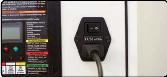
1. Plug the cord set into the side of the incubator and then into the proper outlet.
