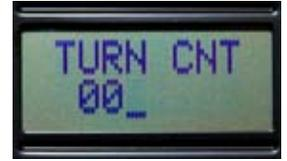
**TURN CNT** - Shows amount of times the turner has turned. Resets at 1000. No count on hatcher models.
