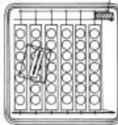
Place eggs in turner with small ends down and adjust temperature as instructed. Place thermometer on top of eggs
