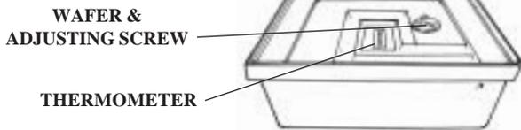
Next, remove the thermometer, and brass thermostat wafer from underneath the liner. Also remove the wingnut and adjusting screw which is under the brass wafer.
