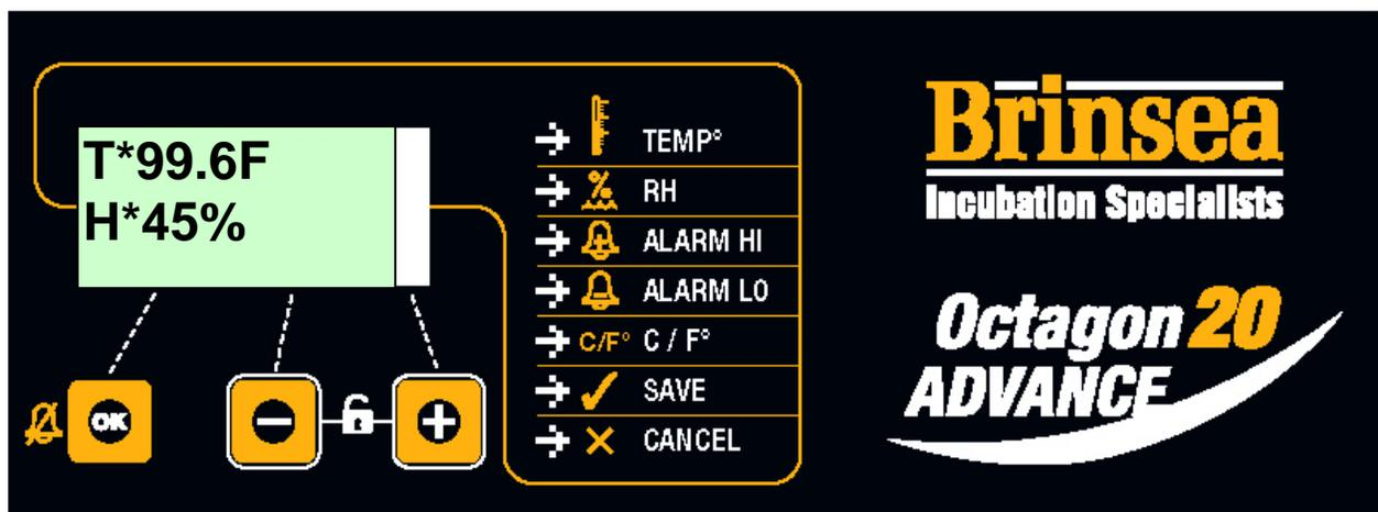
The Octagon 20 Advance control system utilises highly accurate, individually calibrated sensors for temperature and humidity. Be cautious of low cost analogue or digital thermometers and hygrometers when comparing them with the incubator display readings.
